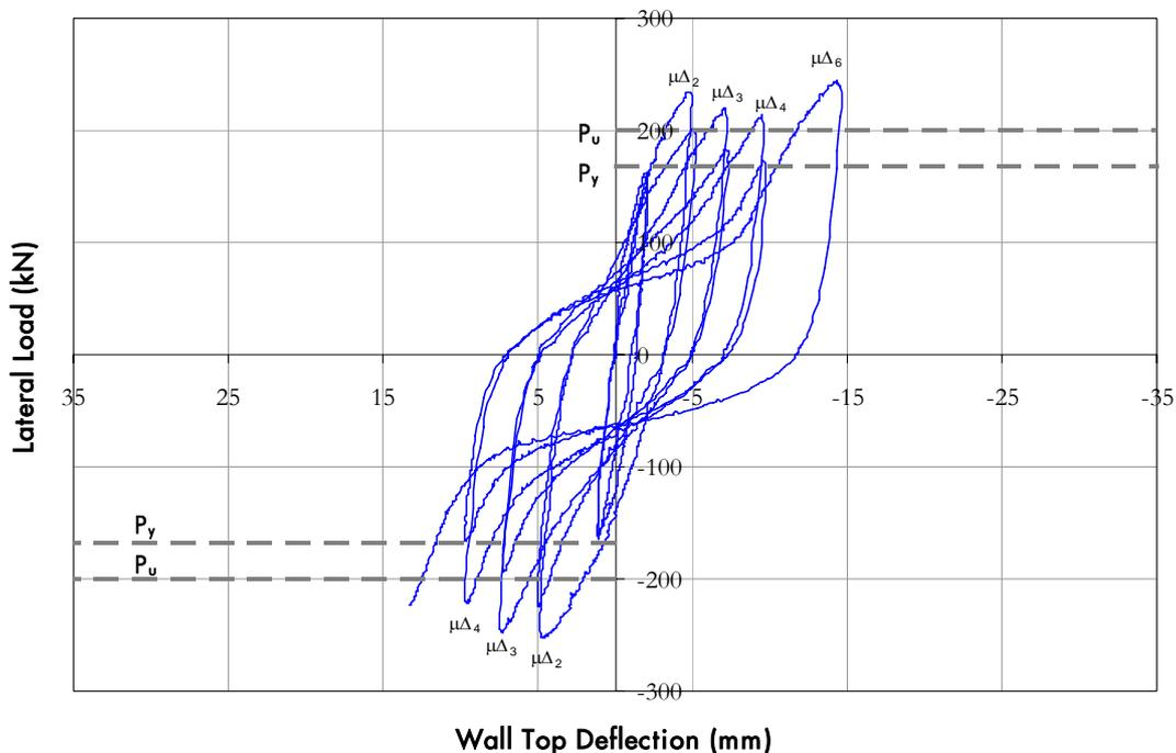
Figure 18 *Load Deflection Performance of test specimen AFS3*
