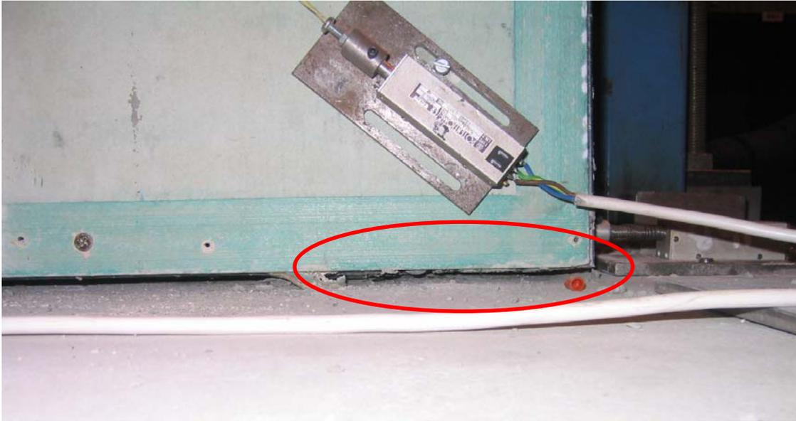
Figure 10 *Crack at the base of AFS1 during load cycles to 200 kN.*
