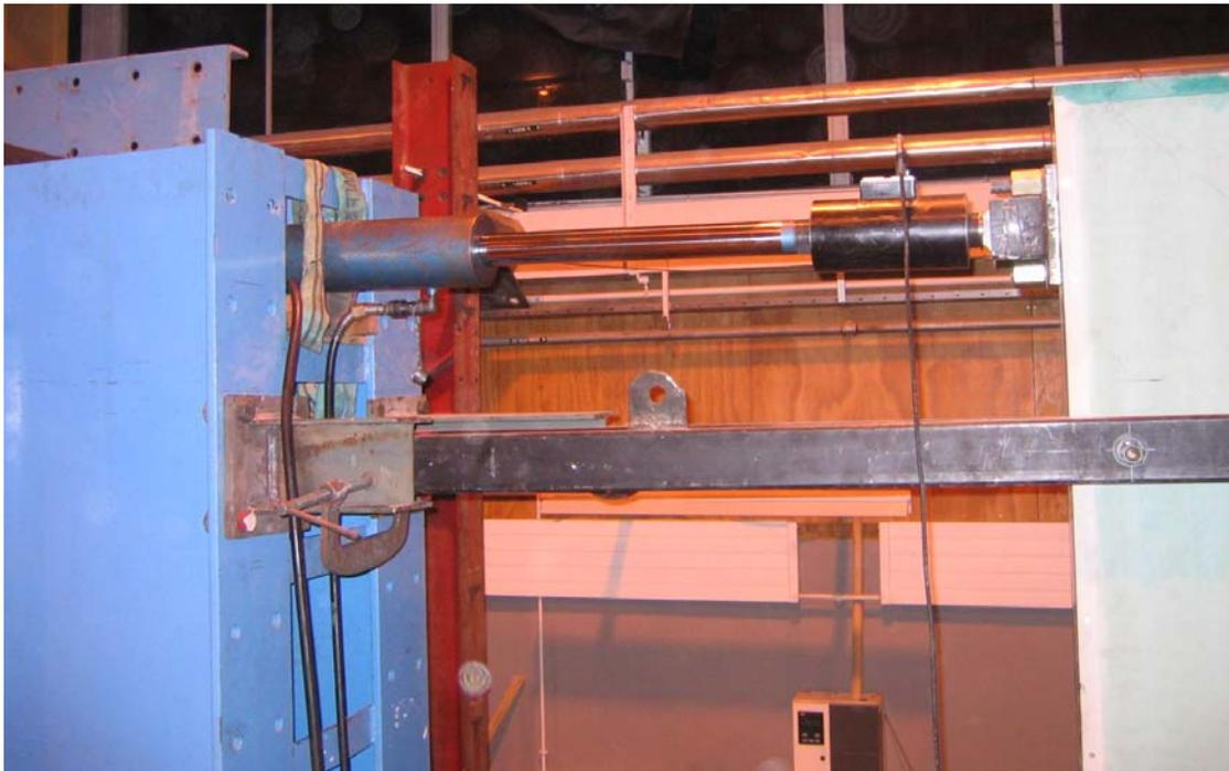
Figure 6 *Connection of the load cell and hydraulic actuator to the AFS150 wall unit*
