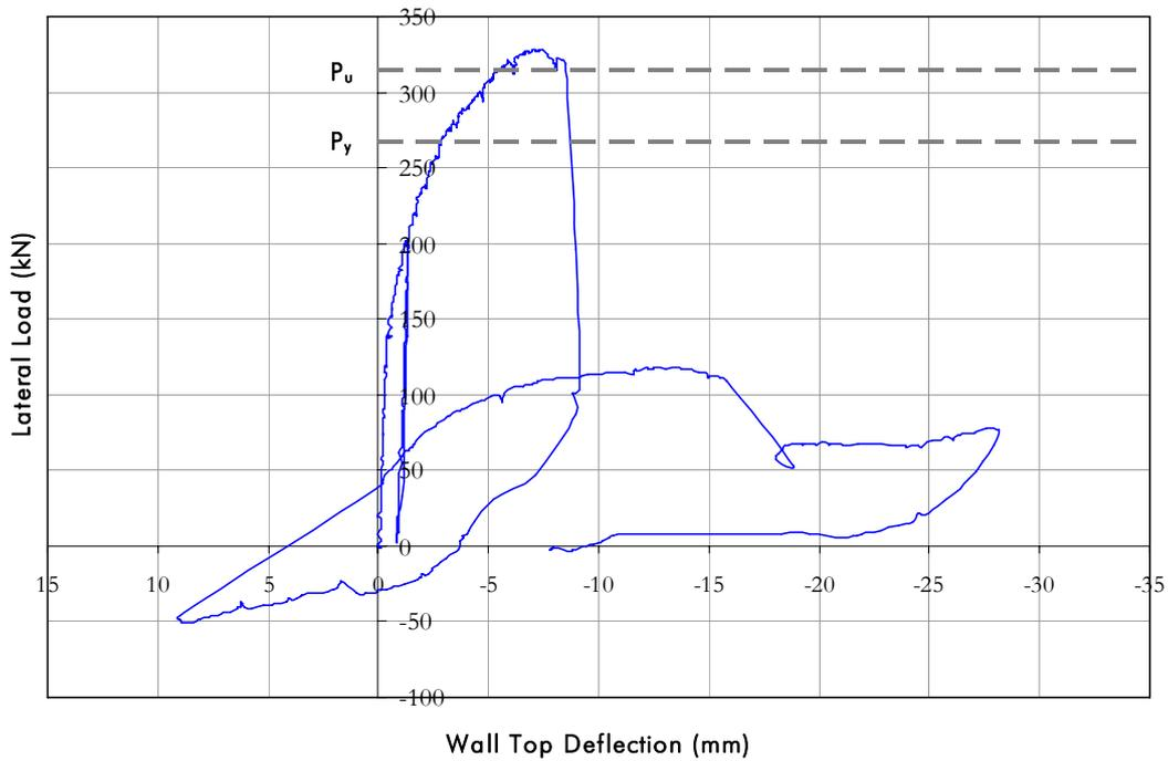
Figure 12 *Load Deflection Performance of test specimen AFS1*
