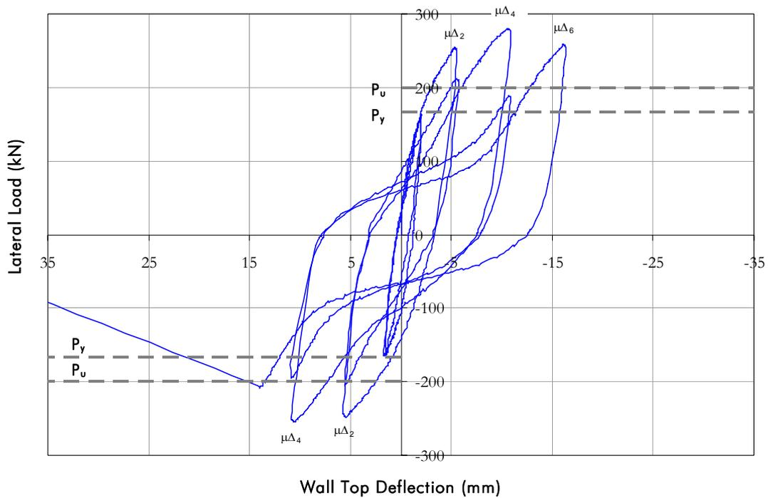
Figure 21 *Load Deflection Performance of test specimen AFS4*
