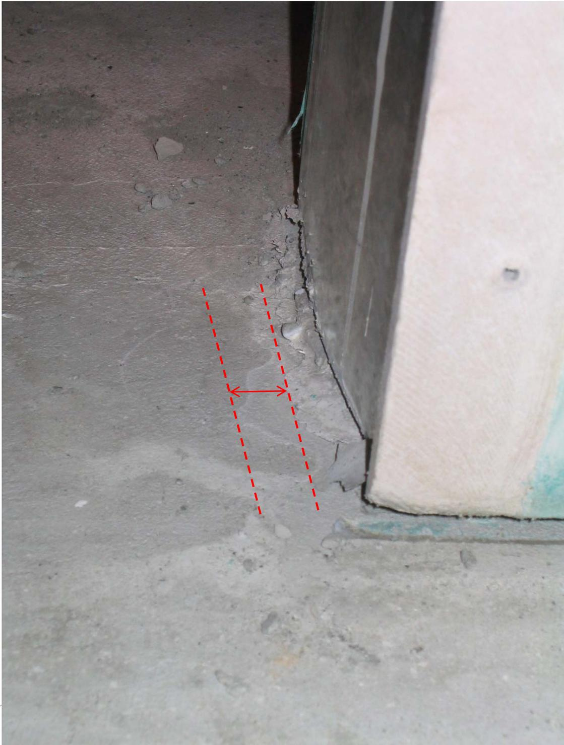
Figure 20 *Measured slip of specimen AFS4 along foundation beam*
