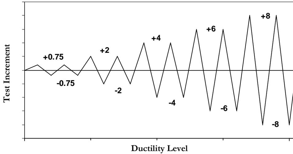
Figure 8 Loading Pattern Applied to the AFS150 Wall Units.
