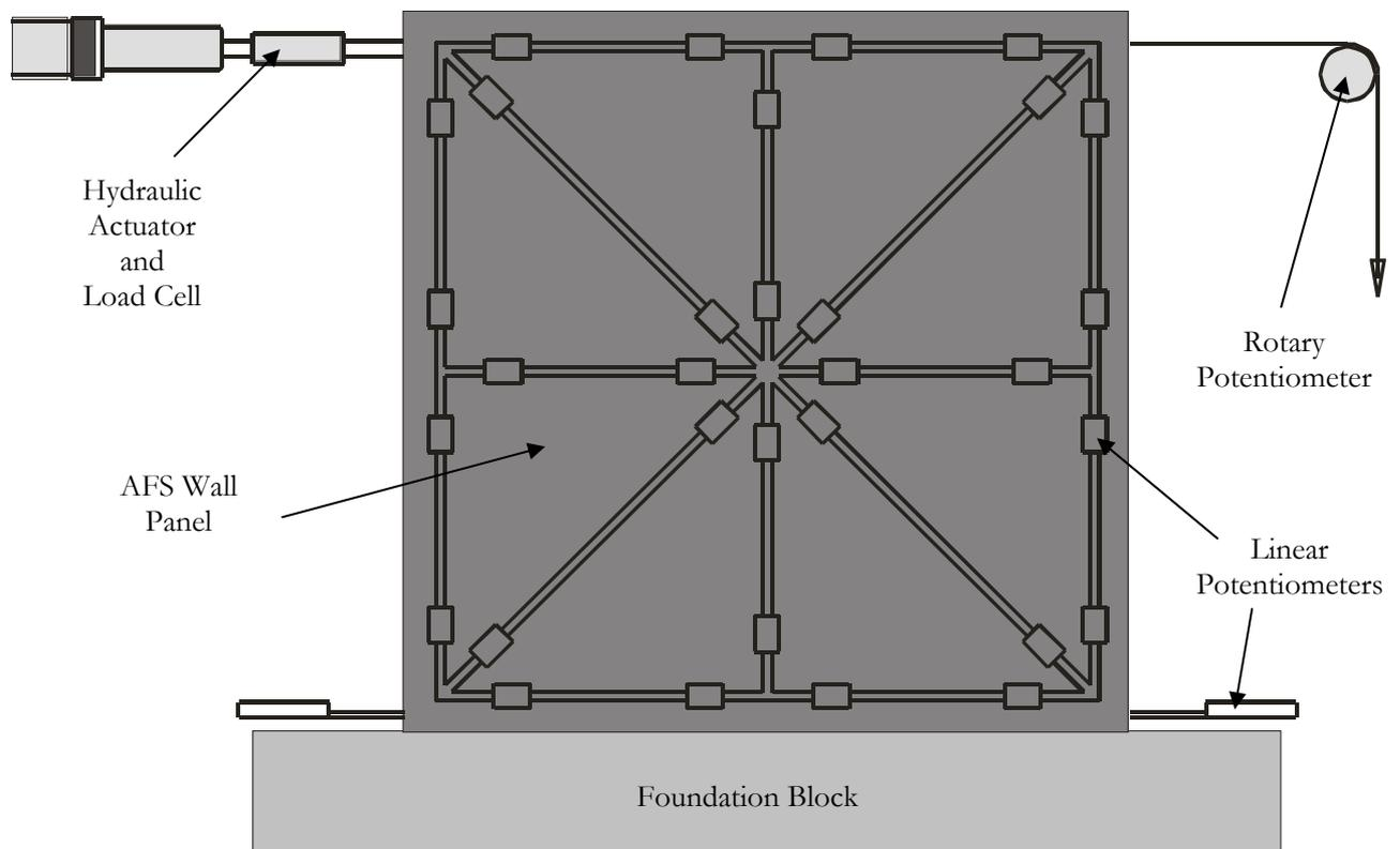
Figure 5 *Instrumentation location on AFS150 wall units*
