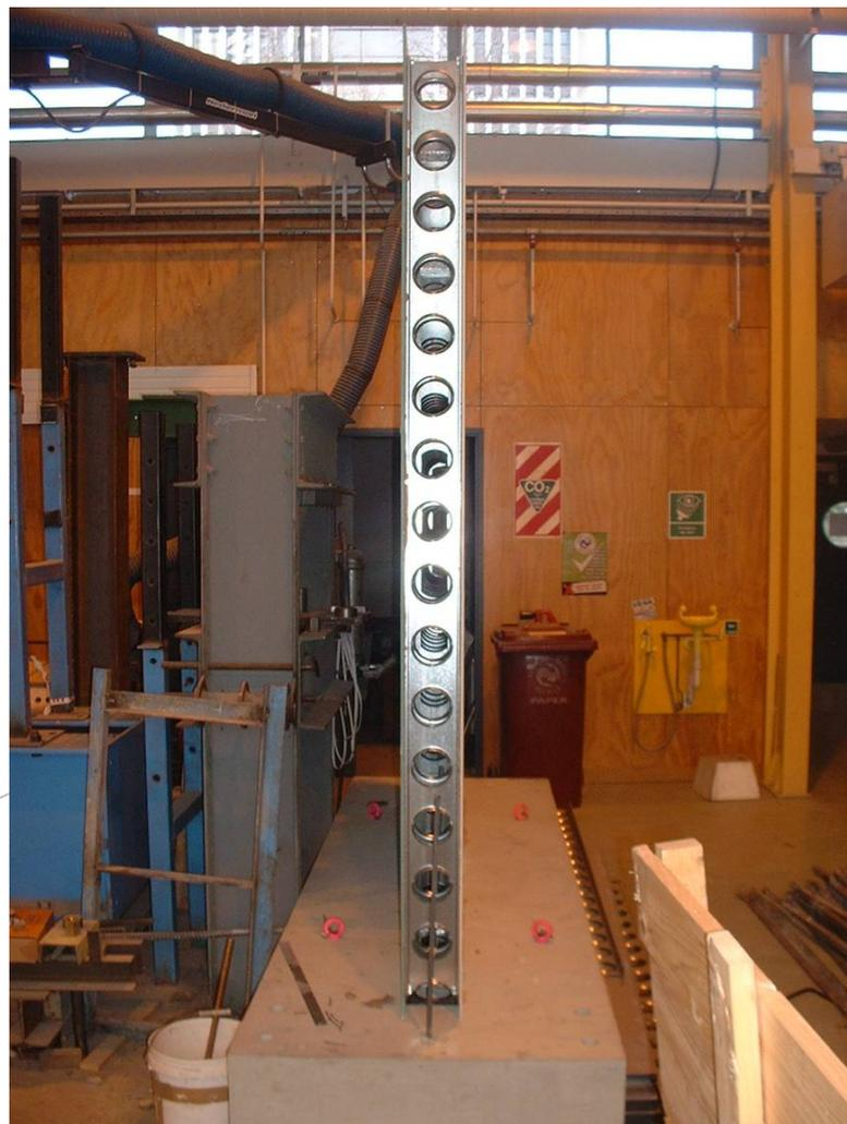
Figure 3 *End view of the panels, showing voids in which the horizontal reinforcing was placed*
