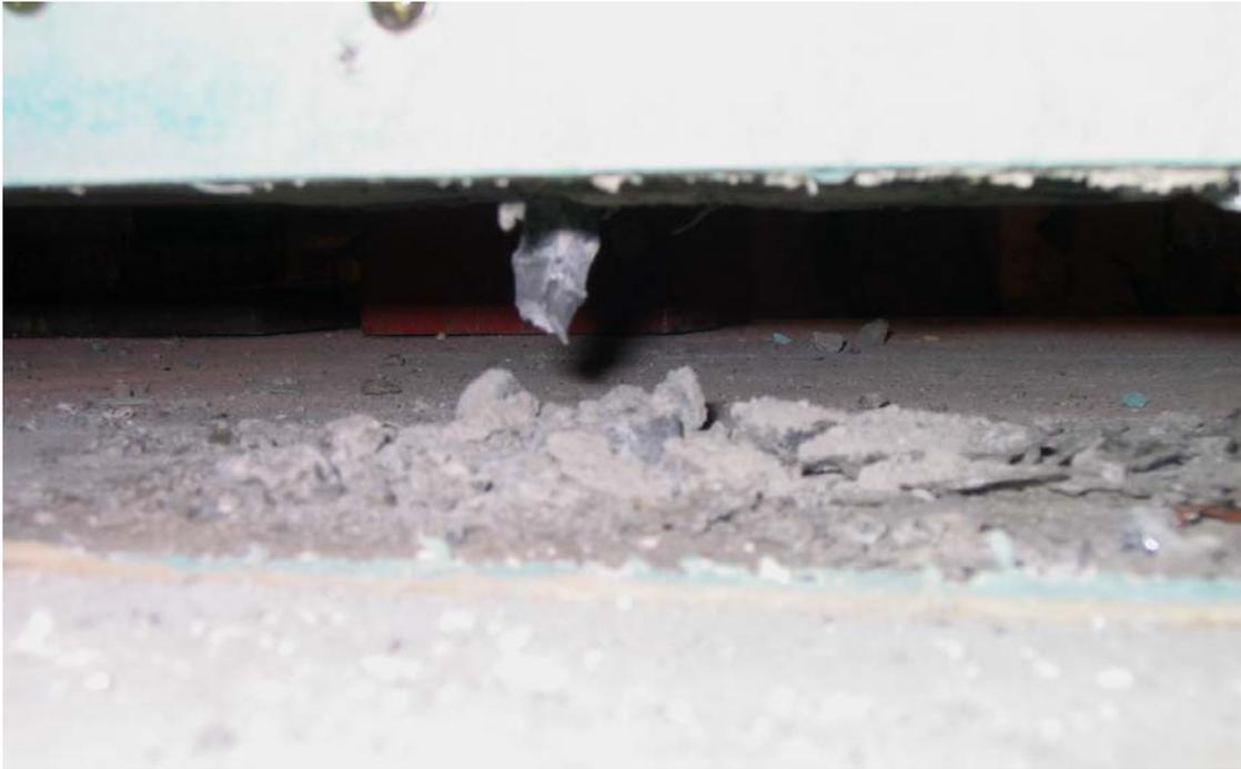
Figure 14 *Fractured reinforcing bar in specimen AFS2*
