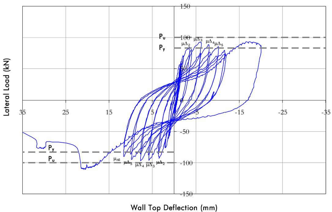
Figure 24 Load deflection performance of test specimen AFS5
