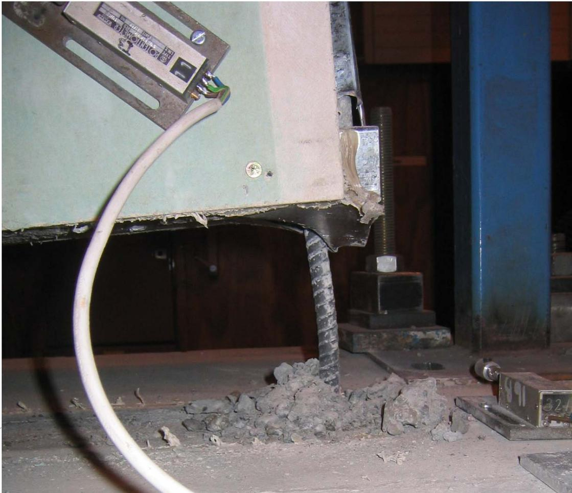
Figure 17 *Bond failure with end reinforcing bar*
