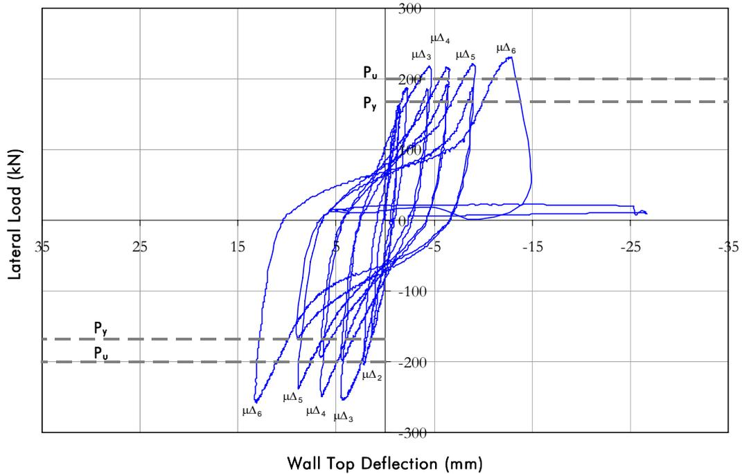
Figure 15 *Load Deflection Performance of test specimen AFS2*
