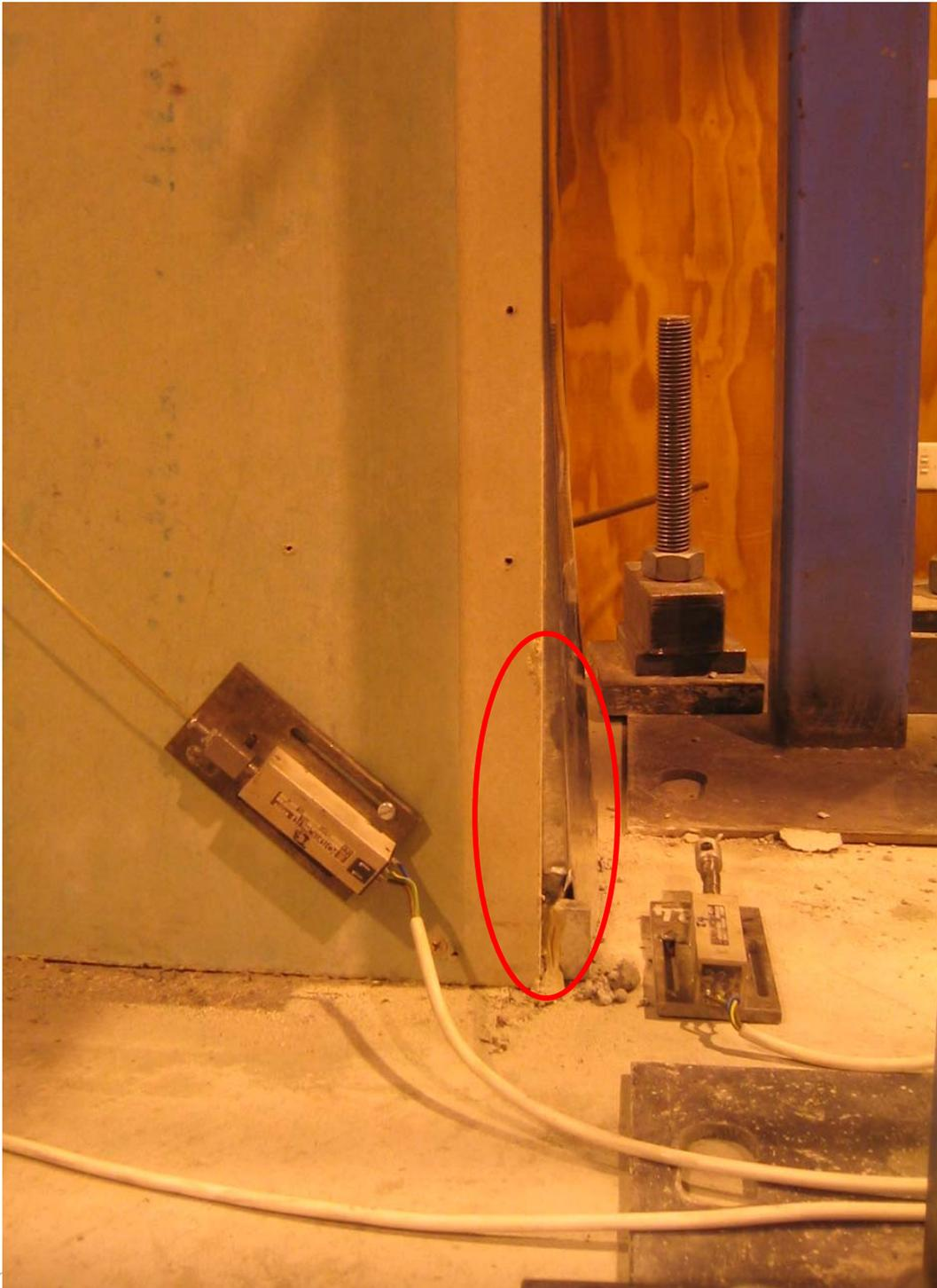
Figure 23 *Expansion of the end plate in test specimen AFS5*
