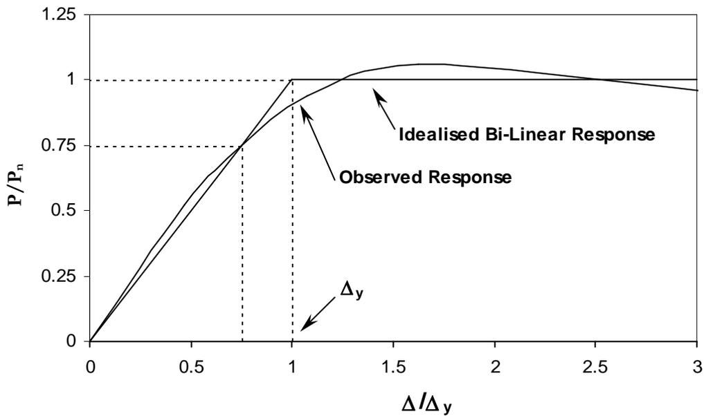
Figure 9 Determination of the Equivalent Bilinear Stiffness and Yield Displacement.
