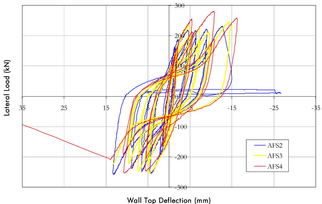
Figure 25 *Load Deflection Performance of test specimens AFS2, AFS3, AFS4*
