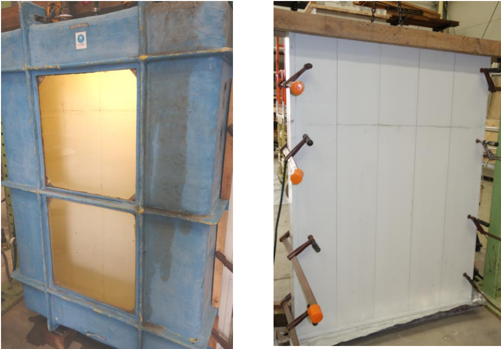
Figure 6 Test chamber fitted to the wall panel
