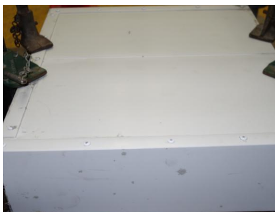
Figure 10 Water permeability test observations of the block specimen under test
