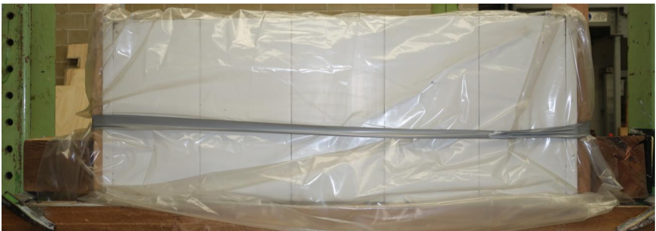
Figure 4 Curing with the use of impervious plastic over the wall panel
