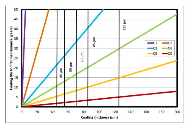
Figure 13: Life to first maintenance of hot dip galvanized steel in ISO 9223 corrosivity categories
