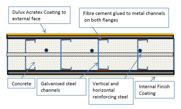
Figure 4: The complete LOGICWALL formwork with reinforcement and concrete
