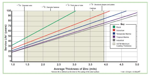
Figure 12: Service life chart for hot-dip galvanized coating in open atmosphere
