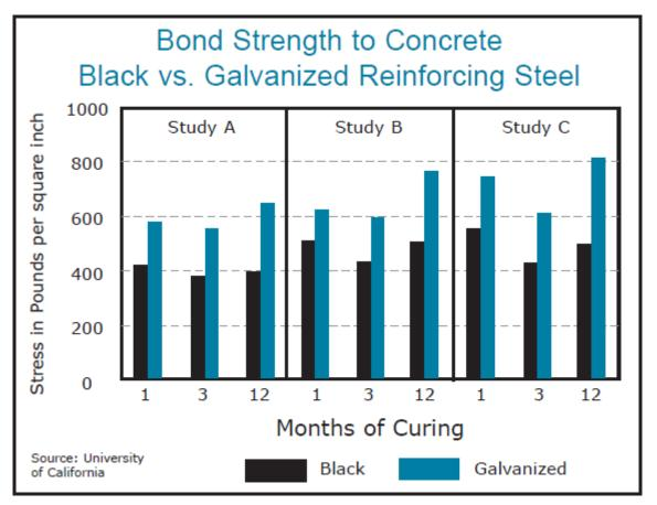
Figure 8: Bond strength to concrete black vs. galvanized reinforcing steel
