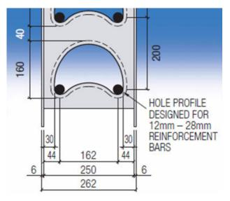
Figure 7: Reinforcement layout and cover provision for the double reinforcement LOGICWALL system
