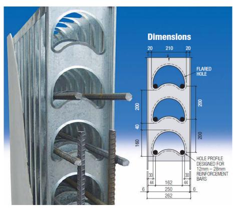
Figure 3: LOGICWALL system with double reinforcement
