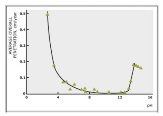
Figure 9A: Penetration of pure zinc due to corrosion as a function of pH
