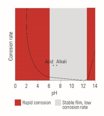
Figure 9B: Zone of stability of galvanized coating in carbonated concrete
