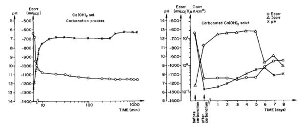
Figure 11: Changes of  $E_{corr}$  and  $I_{corr}$  of galvanized steel during carbonation of alkaline solutions
