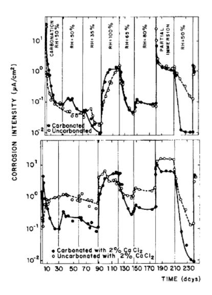
Figure 10: Evolution of  $I_{corr}$  of galvanized reinforcement embedded in carbonated and uncarbonated mortar, with and without chlorides
